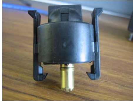
Close up of the EDIS Coil End
