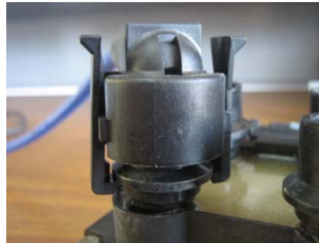
EDIS Assembly showing how the plug wire coil end clips onto the coil tower.
