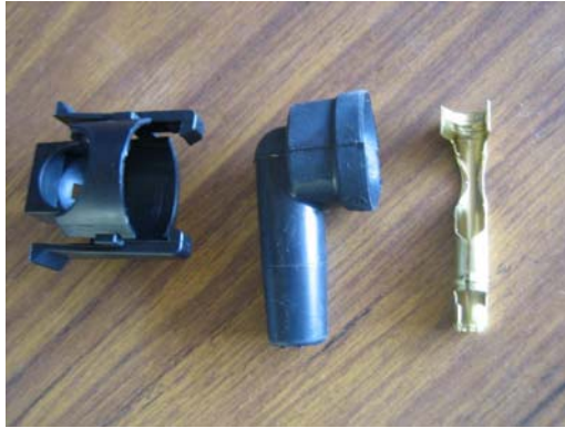
Set out the EDIS conversion kit (Clip, Boot, Terminal).
