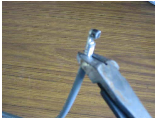
Cut the wire at the base of the old terminal or old boot.
