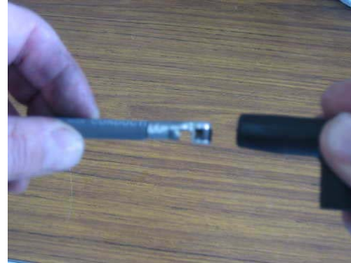
With your original wire in hand, grasp the boot and give it a pull to see if it will come off. If it doesn't, that's ok, we'll cut the wire at the base of the boot.
